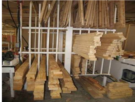
Figure 21 Cut stud rack between wall tables
