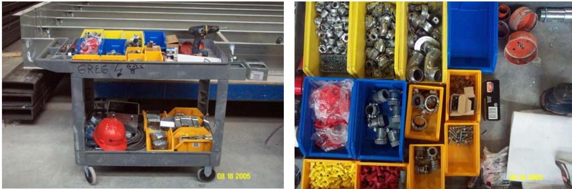
Figure 60 Standardized supply cart for rough electric activities
