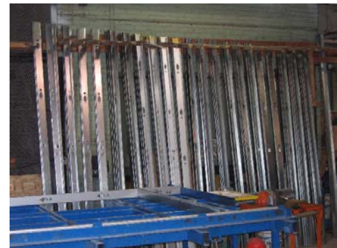
Figure 54 Studs for building sloped wall prepared and stored
