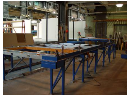
Figure 44 Wall framing station
