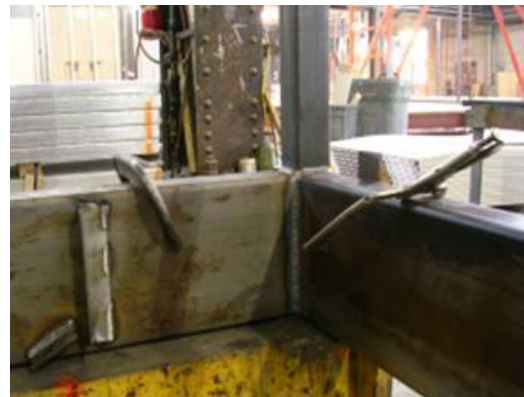
Figure 40 Welded chassis corner
