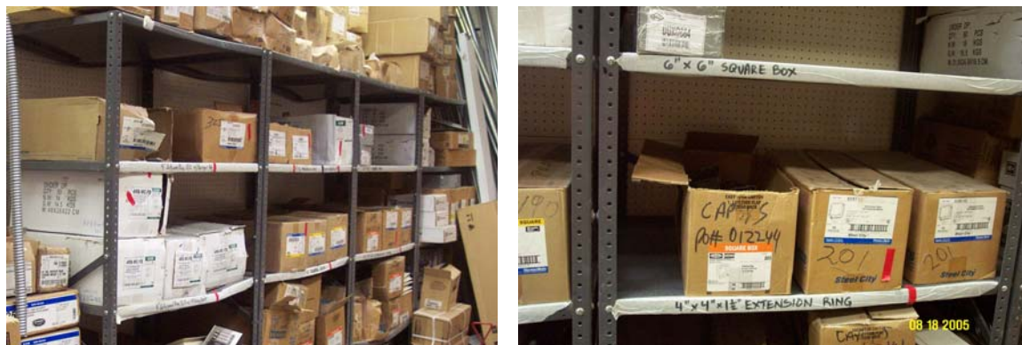
Figure 62 Organized shelving for larger parts: “golden zone” (left) and typical shelf with three cartons, only one of which is open, and red replenishment point marked on shelf
