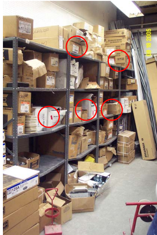
Figure 59 During the RPI event, use of red tape to identify currently used parts (inside circles)
