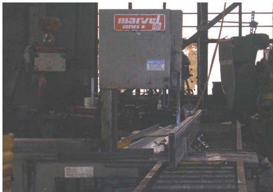
Figure 1. Dull band saw (floor framing)
