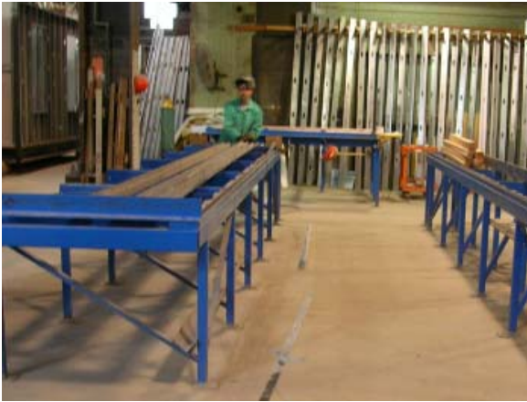
Figure 38. Different length wall studs cut in batches
